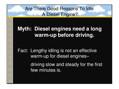
Diesel bus manufacturers suggest a warm-up time of less than 5 minutes. It is considered much more effective to warm-up a diesel bus by driving at a slow, steady speed than to idle for lengthy amounts of time at start-up.
