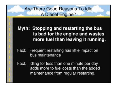
According to most sources, idling for more than 10 second uses more fuel than restarting a school bus diesel engine. Frequent restarting does necessitate more maintenance of mechanical systems but this cost is far less than the combination of additional idling engine maintenance costs and the fuel wasted during idling.
