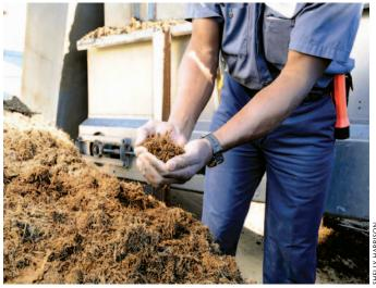
It is prudent action to focus on feedstocks such as agricultural wastes and residues. Here, a Verenium employee handles sugar cane bagasse biomass (residue left after product extraction) to be used at the company's cellulosic ethanol demonstration-scale plant in Jennings, La. Commissioned in May, the facility is the first of its kind in the nation.
