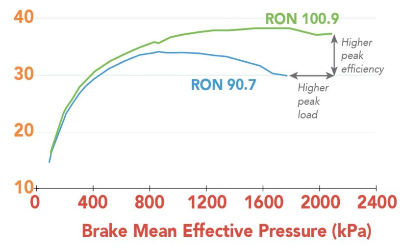
Engine: Ford Ecoboost 1.6L 4-cylinder, turbocharged, direct-injection, 10.1 CR source: C.S. Sluder, ORNL
