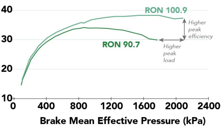
Engine: Ford Ecoboost 1.6L 4-cylinder, turbocharged, direct-injection, 10.1 CR
