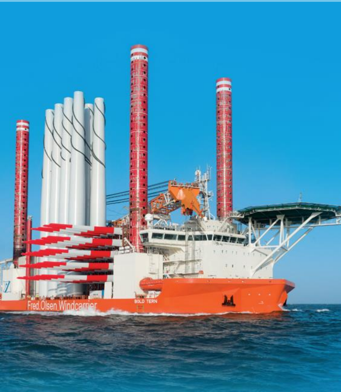
Turbine Installation Vessel
