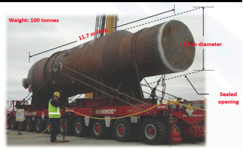
Loaded on a 40-wheel truck; destined to be stored as radioactive waste.
