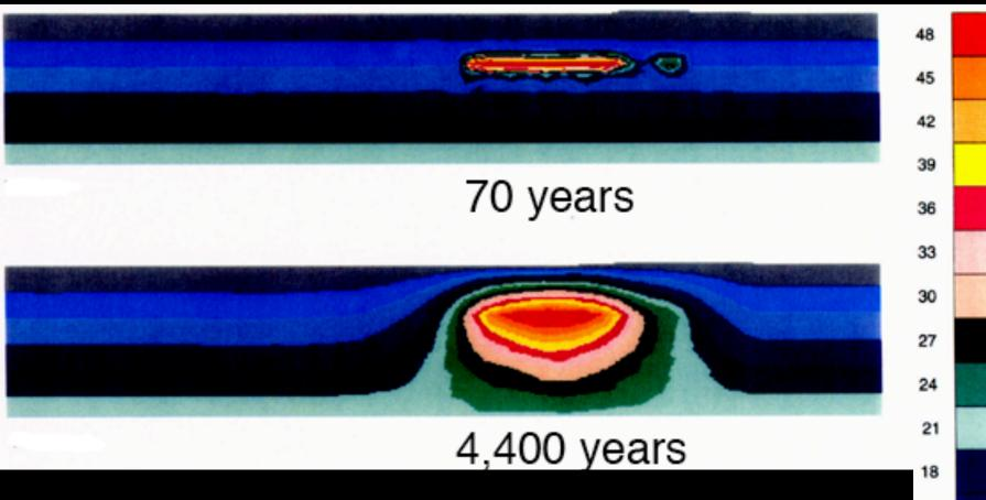
Heat continues to be generated by radioactive disintegration. This heat goes into the rock, raising the temperature.
