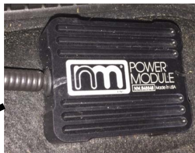
NM Engineering Power Module (PM) intercepts T-MAP sensor and increases boost. PM installed by previous owner; PM was disconnected for all tests except these final E25 WOT tests.
