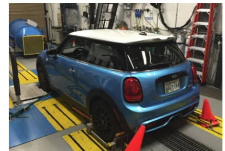
2006 Dodge Charger dynamometer settings used with Mini Cooper vehicle to simulate downsizing
