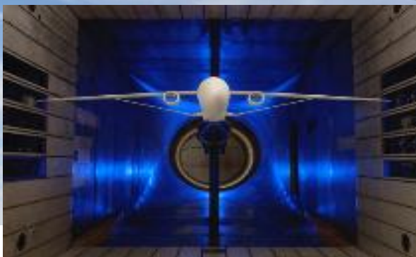
Transonic Truss-Braced Wing 7%-10% fuel burn benefit
