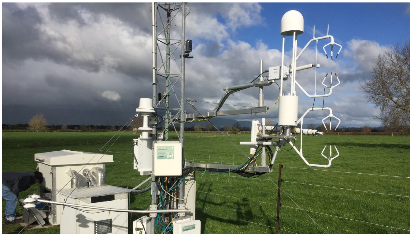
An Eddy Covariance (EC) tower measuring carbon dioxide ( \text{CO}_2 ), methane ( \text{CH}_4 ), nitrous oxide ( \text{N}_2\text{O} ) and water using two different analysers for comparison.
