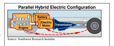
and the combustion engine power the transmission. In addition, through a process called *regenerative breaking*, energy lost due to braking is recovered and utilized to charge the battery.
