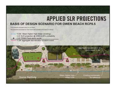
The result of this exercise: a complete reworking of the project and now the design clearly indicates a sea level projection, and any facilities that could be potentially impacted at a future date have been moved upland in the design.
